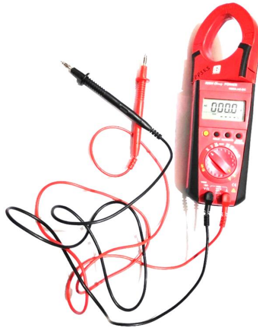
Picture 3 RISH POWER CLAMP 1000 A/400 A AC-DC
