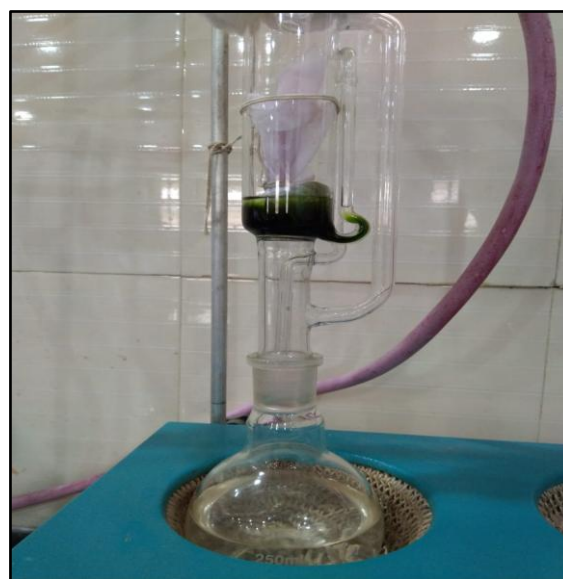
Figure : Soxhlet extraction
