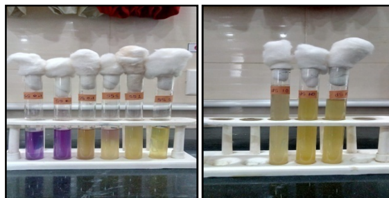
Figure : Result of MPN before addition of coagulant in borewell water sample
